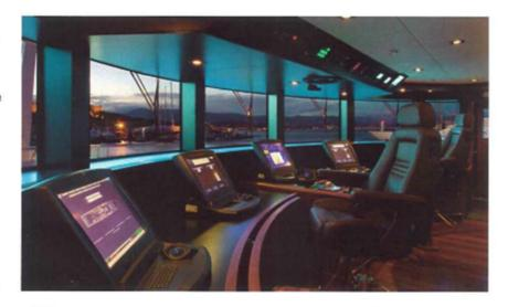
I have installed two Recaro Navigators into the bridge of M/Y Maraya (above). They covered them with the leather of our choice, which in this case ended up as Fendi. I also installed the Kelvin Hughes Ergo Pods in the armrest to control the integrated bridge equipment, which seems to have worked out well.
