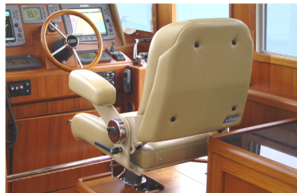
Cabinet space with a view! Top: Two 500N Slimlines with deck penetrating telescoping pedestals aboard an MJM 34Z. Right: The helm of the Grand Banks 55 Eastbay SX features a deck penetrating pedestal which provides an adjustable seat height for better visibility.
