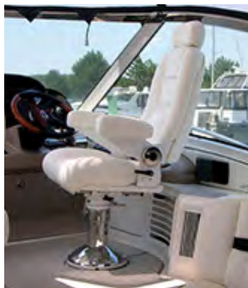
Above left: a 52 SeaRay Sedan Bridge refit with a 500NXH -3NF in "White" UltraLeather. The installation was easy thanks to our 6-bolt to 8-bolt adapter plate. (see page 15).
