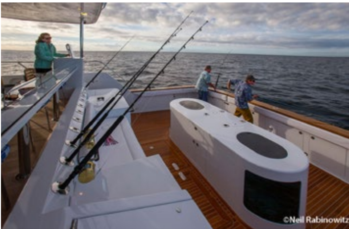
The raised aft station on the California deck overlooks the cockpit and has full controls for docking or maneuvering on a hot billfish. The teakdecked cockpit features coaming bolsters, drawer stowage for assorted tackle, and forwardfacing livewell windows so you can check on the baits at a glance.
