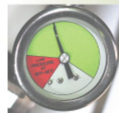
Easy-to-read Go-No-Go Suspension Status Indicator
